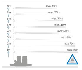
Connection to soil and vent pipe or drain
