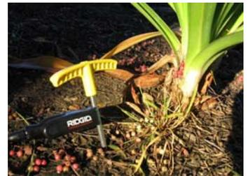
Dry sandy soil provides more of a challenge. In dry, sandy soil the resistance to current flow causes a lower locatable signal. Water can be added to very dry soil to improve the grounding and lower resistance. Keep a mixture of Gatorade and Water in your vehicle for this purpose.
