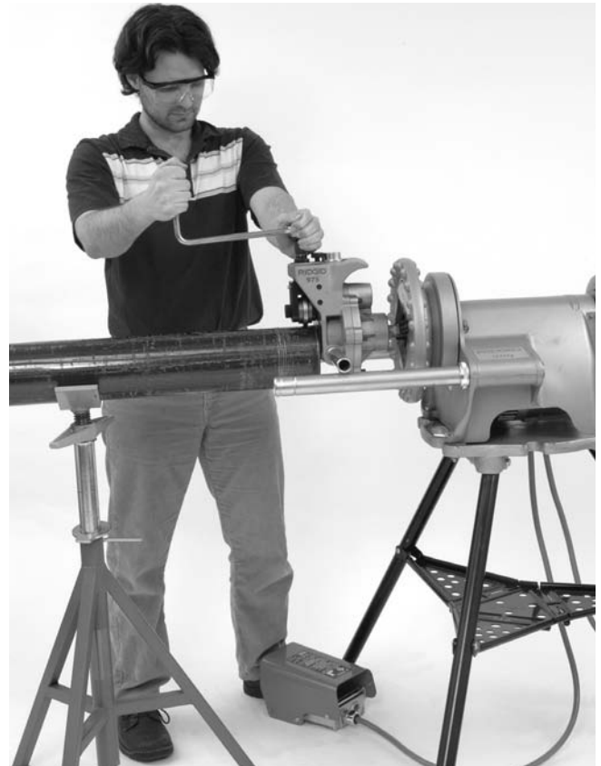
Figure 12 – Roll Groover Operating Position
