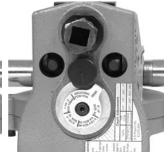
Figure 15B – Gauge In Grooving Position
