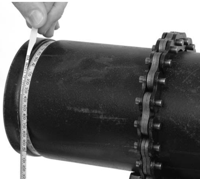
Figure 11 – Checking Groove Diameter With A Diameter Tape
