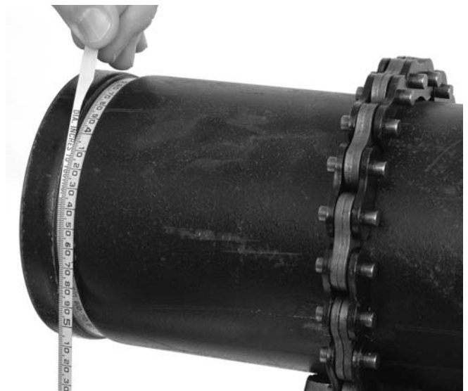
Figure 16 – Measuring The Groove Diameter With A Diameter Tape
