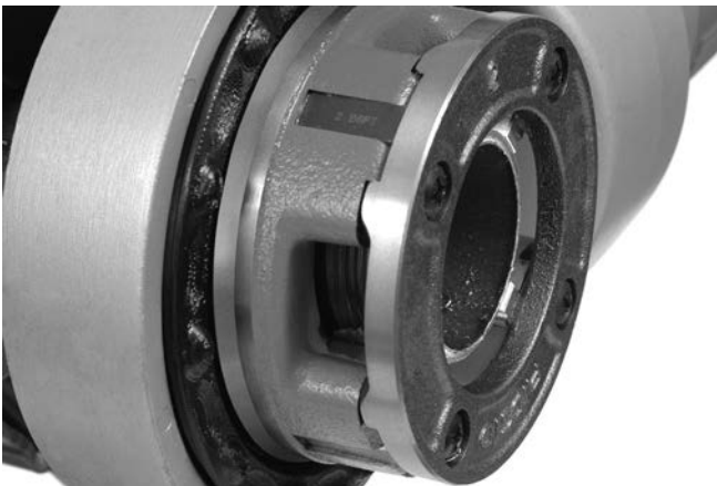
Figure 15 – Pipe Even with Edge of Dies
