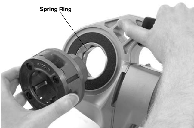
Figure 9 – Installing Die Heads into 600-I Power Drive
