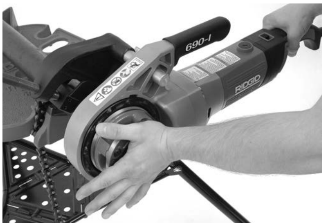
Figure 13 – Entamer le filetage
