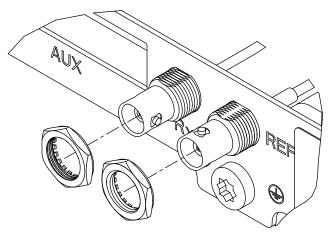
4 Remove the ground screw located below the REF connector with a T30 Torx driver.
