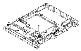
4 Remove the Power Amplifier Module from the Repeater.
