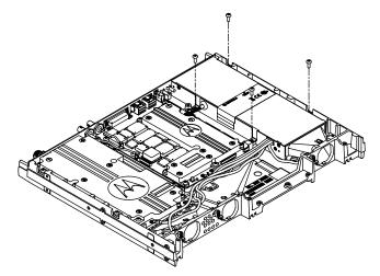
2 Remove the Power Supply Module from the repeater.
