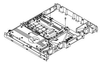
**3** Remove the Modem from the repeater.
