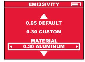
This setting tells the Thermal Imager what surface material it is measuring. This is important, because setting the right emissivity has a significant effect on the accuracy of temperature readings.
