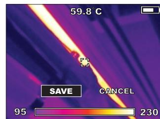
To write the image to SD card, press the button on the arrow keypad or pull the trigger again. Or, to discard the image, press the arrow button to highlight CANCEL, then press the button.
