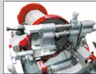
Blade-type cutter on N100A
