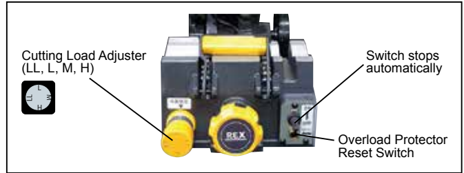
Fig.1 All cutting operations located at the front
