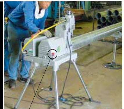
Raise the red knob on the head lock pin to release the self-centering head.
