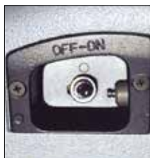
Switch protects die head from touching hand wheel
