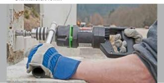
Hand-held drilling machine EHB 16/2.4 S R/L
