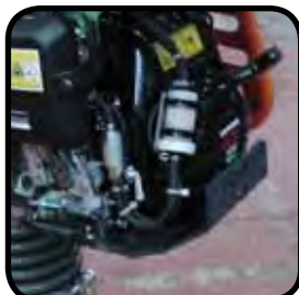
Duel Fuel Filtration system
