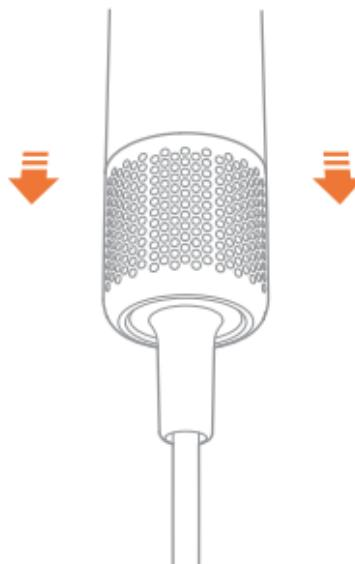
**⚠** Do not rinse the stainless steel filter with water, as this may cause it to not work correctly.
