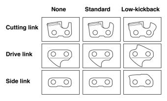
Combining these links in different ways gives different degrees of kickback reduction. In terms of kickback reduction alone, four different types of link are available.
