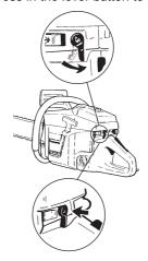
Note: It is not necessary to pump continuously. When the extra oil flow has been activated oil consumption increases by 40-80%, depending on the oil pump's basic setting.
