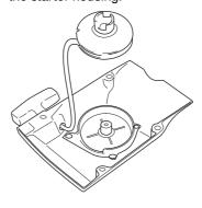
Remove the recoil spring by tapping the starter, with the inside facing downwards, gently on a work bench. If the spring pops out during assembly, coil it up from the outside, working inwards.
