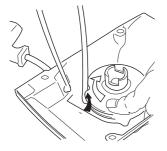
Undo the screw in the centre of the pulley and remove the pulley. Insert and fasten a new starter cord to the pulley.
