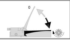
The left-hand lever is used to operate the sweeper brush mechanism.
