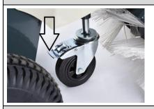
Brake on: Push the lower lever down
