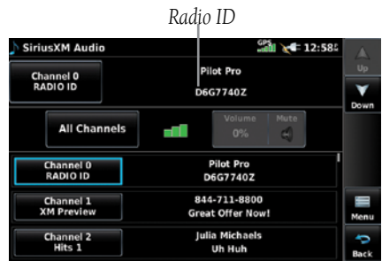
Accessing the SiriusXM Radio ID (Channel 0)
