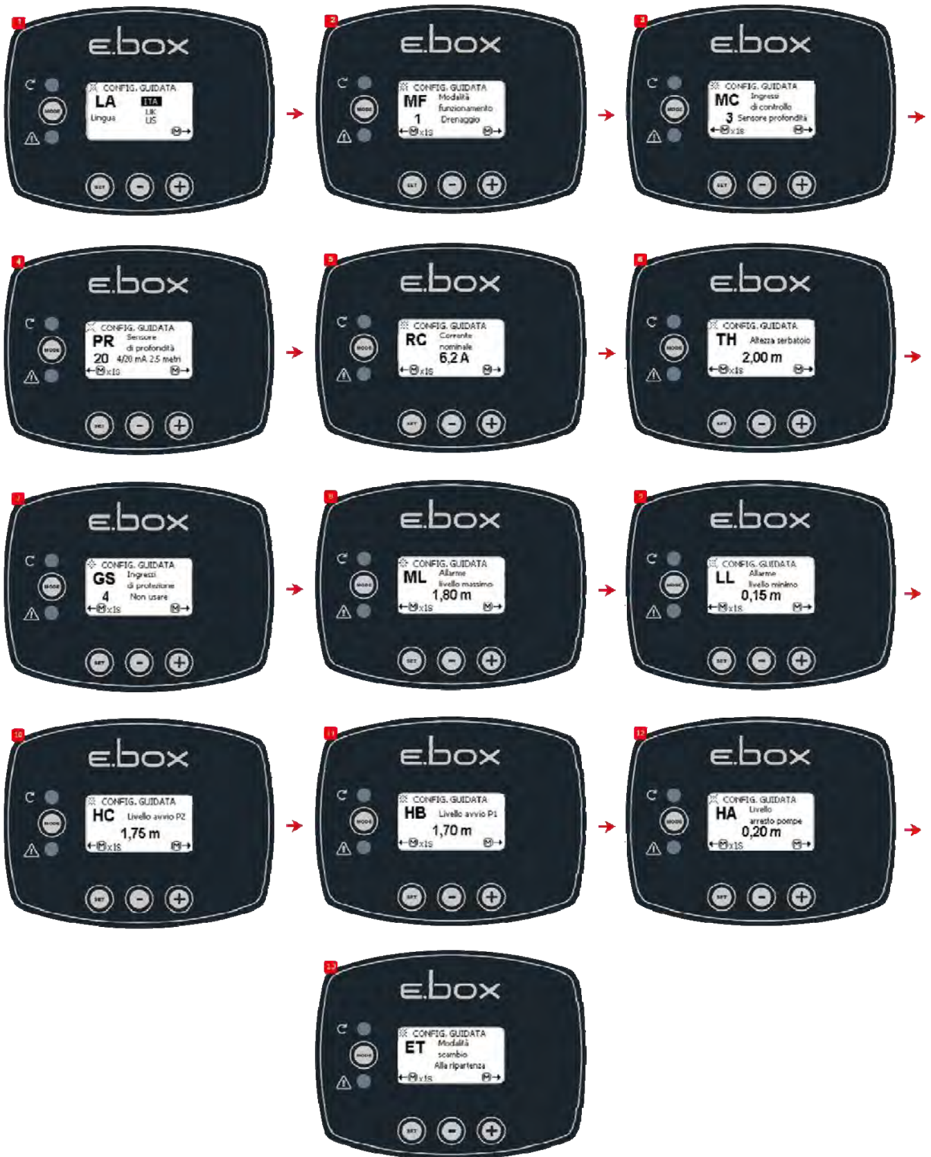
Figure 38: Configuration with only a depth sensor
