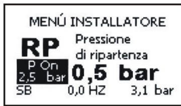
Figure 19: Setting the restart pressure
