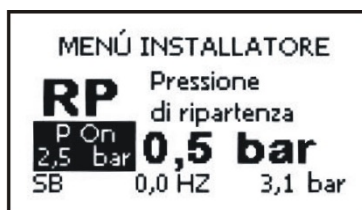
Figure 18: Setting the restart pressure
