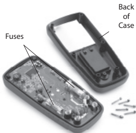
Figure 9 – Removing Back of Multimeter Case
